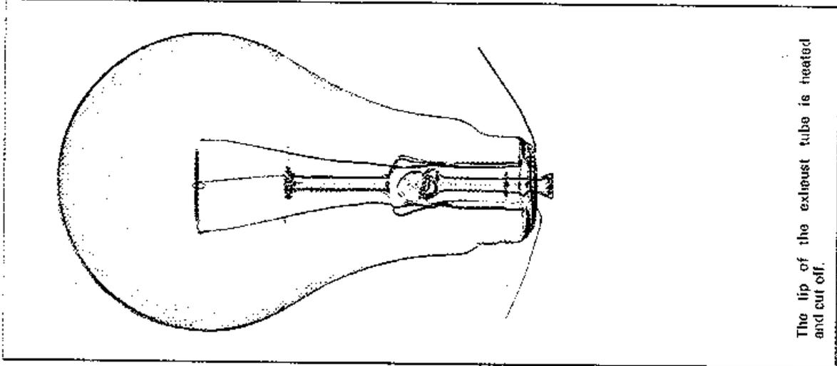
The lip of the exhaust tube is heated and cut off.
