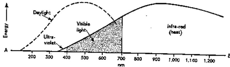
Fig. 2 Spectral power distribution of a gas-filled incandescent lamp
