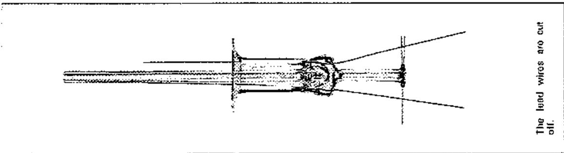
The lead wires are cut off.
