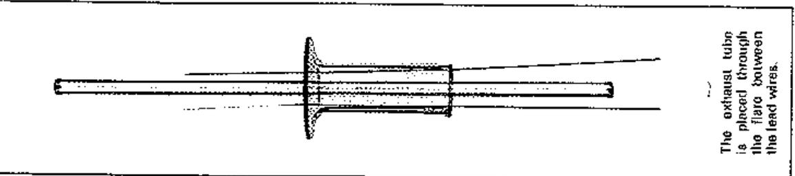
The exhaust tube is placed through the flare between the lead wires.
