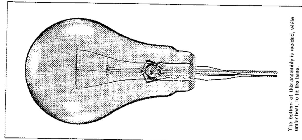
The bottom of this assembly is welded, while under heat, to fit the base.
