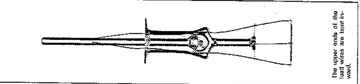
The upper ends of the lead wires are bent inward.
