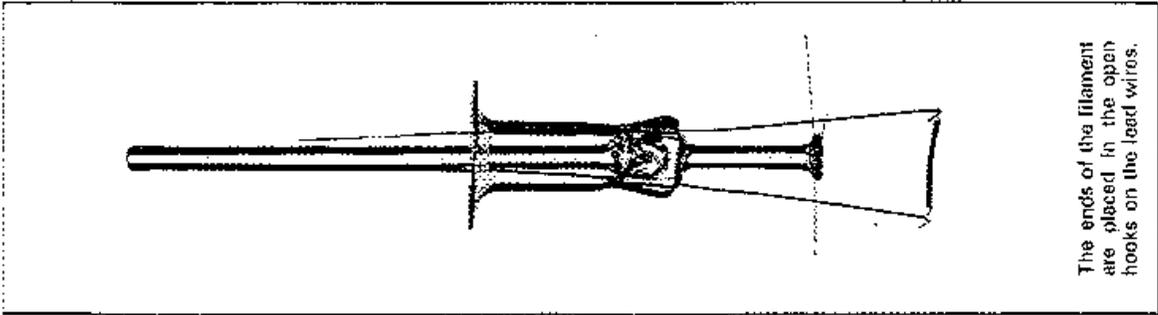
The ends of the filament are placed in the open hooks on the lead wires.
