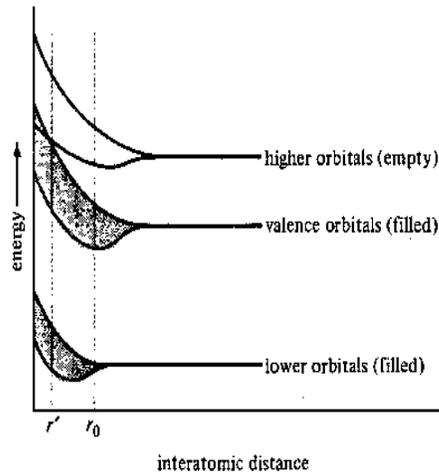
Fig. 3 Energy Bands in a Metal (ABOVE) AND AN INSULATOR (BELOW).
