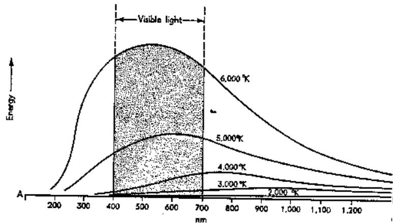
Fig. 1 Spectral power distribution of black body at various temperatures
