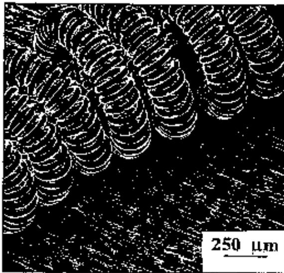
*Figure 4 An example of a coiled-coil filament used in most incandescent lamps today. This figure shows an SEM micrograph of a section of filament that has been removed from the lamp.*
