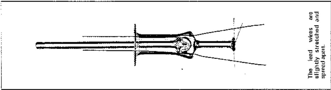
The lead wires are slightly stretched and spread apart.
