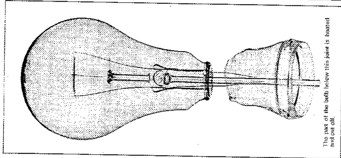
The part of the bulb below this joint is heated and cut off.
