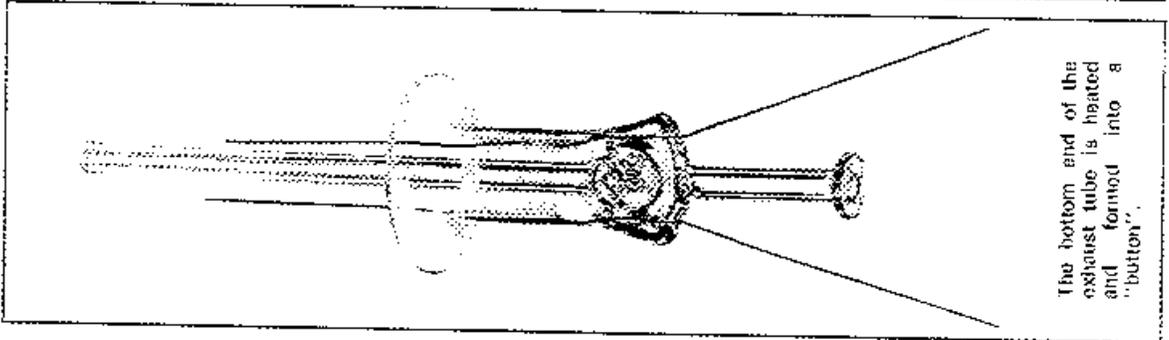
This completes the stage of the assembly which is called the "stem".
