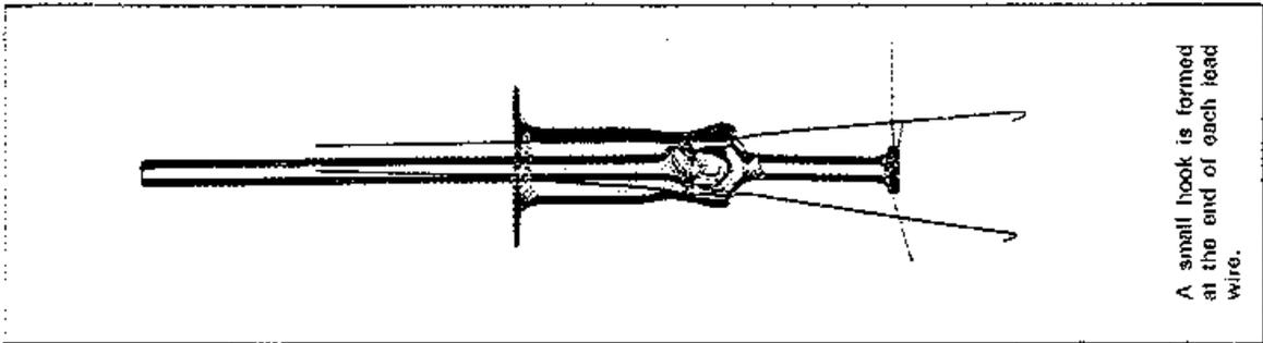
A small hook is formed at the end of each lead wire.
