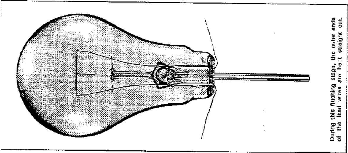
During this flushing stage, the outer ends of the lead wires are bent straight out.
