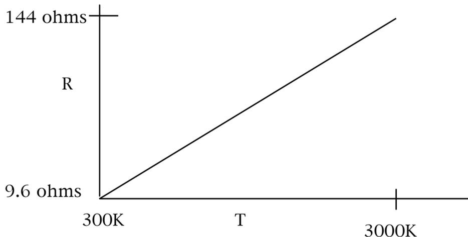
4. From 2, values of  $R$  vs time were measured. From 3, values of  $R$  vs  $T$  were determined. Using these two data sets, values of  $T$  vs time (the filament cooling curve) can be determined.
