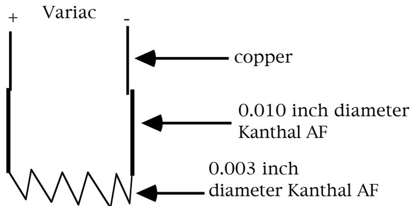
The electrical resistivity of the Kanthal AF wire is  $1.4 \times 10^{-4}$  ohm-cm at essentially all temperatures. This is quite different than the behavior of pure metals such as copper or tungsten, where the electrical resistivity increases significantly as the temperature increases. Have your students determine the electrical resistance of the Kanthal AF wire filament by calculation (using equation 4) and by measurement with the ohmmeter.
